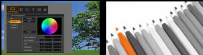
Displays only the color being adjusted; others are displayed in black and white.
